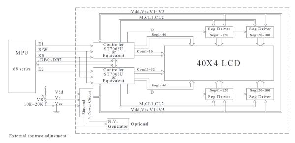
Crystalfontz recommends allowing field adjustment of  $V_0$  for all designs. The optimal value of  $V_0$  varies with temperature, variations in  $V_{DD}$ , and viewing angle.  $V_0$  will also vary module-to-module and batch-to-batch due to normal manufacturing variations. If exposing adjustments to  $V_0$  is not possible, Crystalfontz recommends enabling adjustment of  $V_0$  as part of a product's final test.
