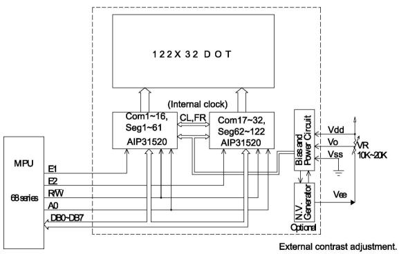
Crystalfontz recommends allowing field adjustment of  $V_0$  for all designs. The optimal value of  $V_0$  varies with temperature, variations in  $V_{DD}$ , and viewing angle.  $V_0$  will also vary module-to-module and
