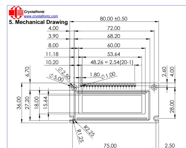
CFAG12232J1-TFH-TJ Display Module Datasheet Release Date 2024-04-16
