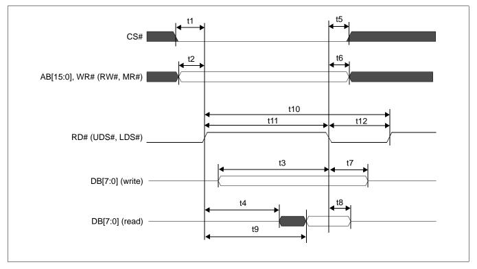
Figure 7-7 M6800 Family Bus Indirect Interface Timing
