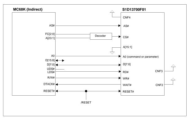
Figure 3-3 Indirect MC68K to S1D13700F01 Interface Example
