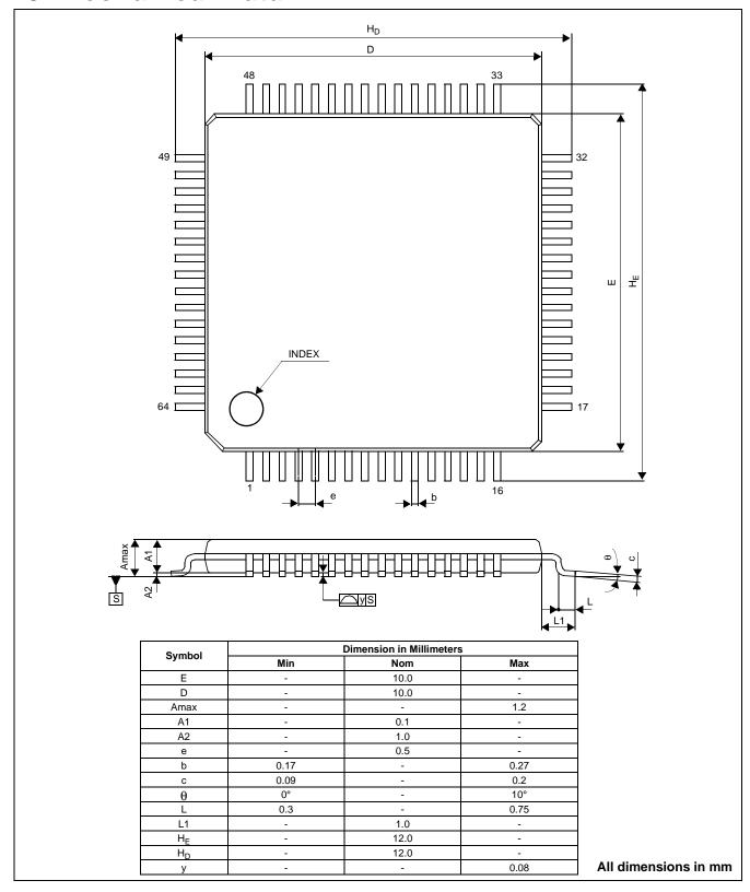
Figure 18-1 Mechanical Drawing TQFP13 - 64 pin
