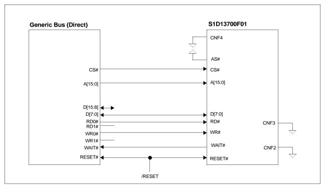
Figure 3-2 Direct Generic to S1D13700F01 Interface Example
