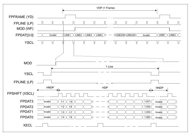
Figure 7-8: Monochrome 4-Bit Panel Timing
