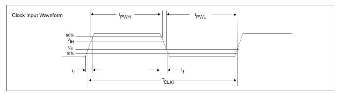
Figure 7-1 Clock Input Requirements
