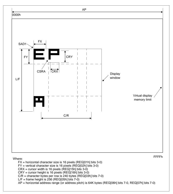
Figure 12-12 Virtual Display (Display Window to Memory Relationship)
