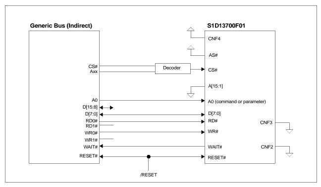
Figure 3-1 Indirect Generic to S1D13700F01 Interface Example
