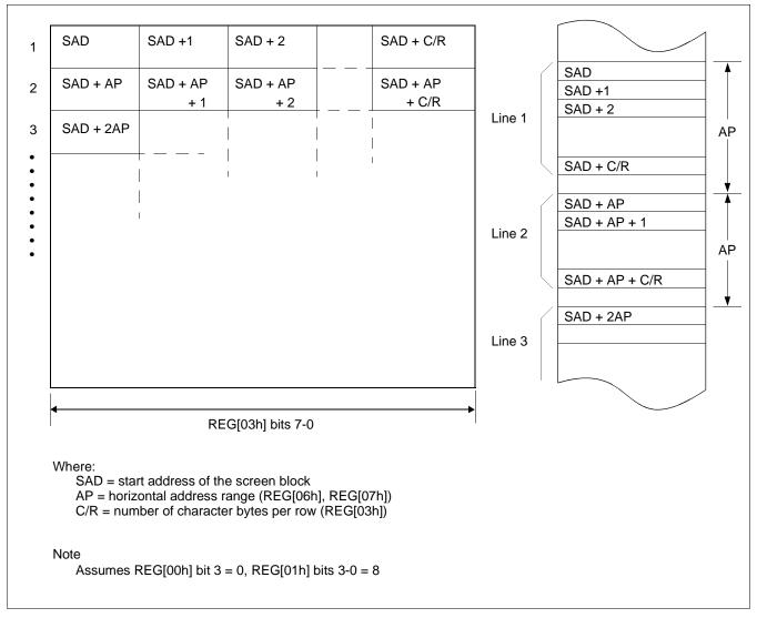
Figure 12-5 Display Addressing in Graphics Mode Example
