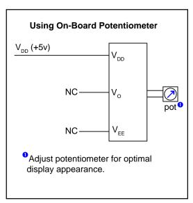
Figure 3. Typical V<sub>O</sub> Connections (External Control or On-Board Potentiometer)
