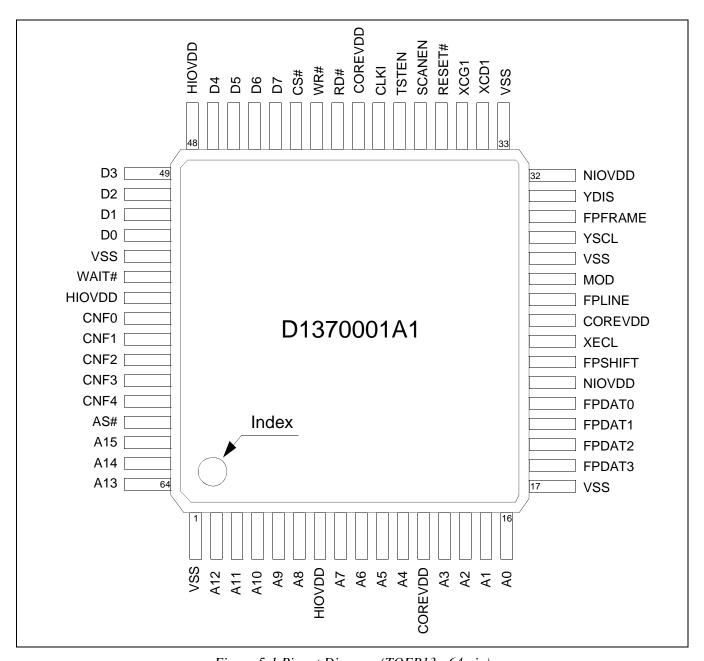
Figure 5-1 Pinout Diagram (TQFP13 - 64 pin)
