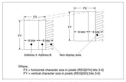
Figure 10-4 Horizontal and Vertical Character Size Example
