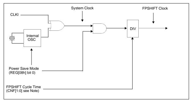
Figure 9-1: Clock Diagram
