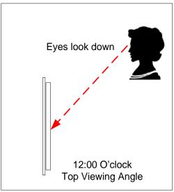
Figure 8. Definition of 6:00 O'Clock and 12:00 O'Clock Viewing Angles
