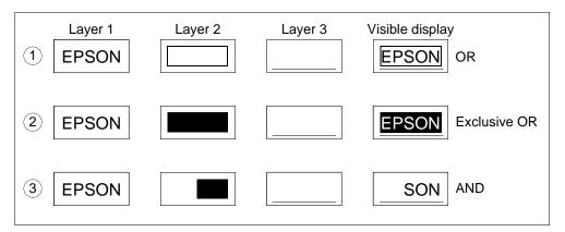
Figure 10-9 Combined Layer Display Examples
