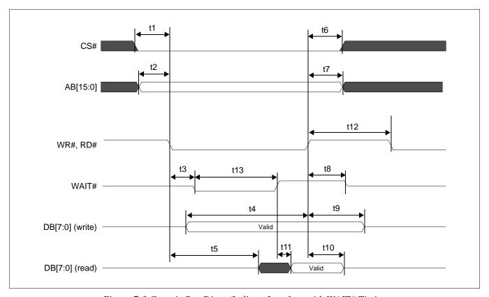
Figure 7-3 Generic Bus Direct/Indirect Interface with WAIT# Timing
