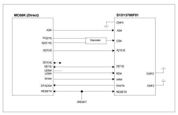
Figure 3-4 Direct MC68K to S1D13700F01 Interface Example
