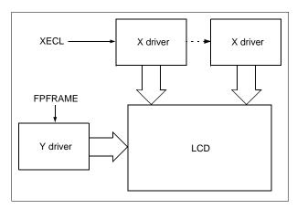
Figure 10-2 Single Drive Panel Display
