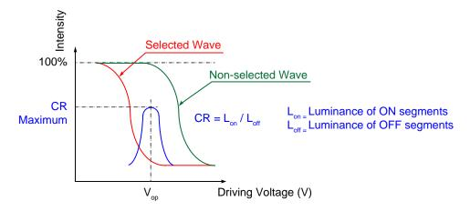
Figure 5. Definition of Operation Voltage (V<sub>OP</sub>)
