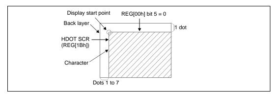
Figure 10-1 Screen Origin Compensation and HDOT SCR Adjustment
