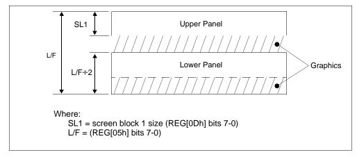
Figure 10-6 Dual Panel Display Height
