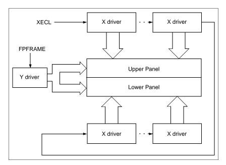
Figure 10-3 Dual Drive Panel Display
