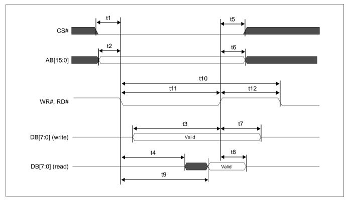
Figure 7-4 Generic Bus Direct/Indirect Interface without WAIT# Timing
