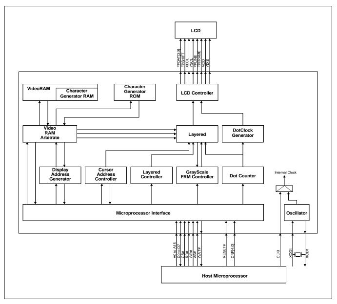
Figure 4-1 Functional Block Diagram
