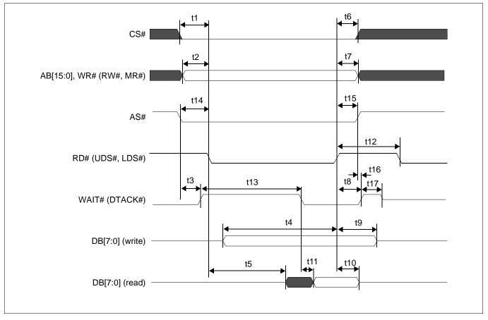
Figure 7-5 MC68K Family Bus Direct/Indirect Interface with DTACK# Timing
