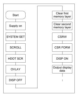
Figure 15-1 Initialization Procedure
