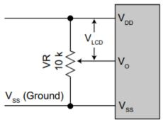
Although a potentiometer is shown as a typical connection,  $V_0$  can be driven by a microcontroller, using either a DAC or a
