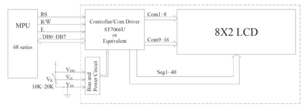
Set V<sub>0</sub> to +1v such that  $V_{LCD}$  = +4v as an initial setting. Using the potentiometer VR, adjust V<sub>0</sub> for optimal display appearance.
