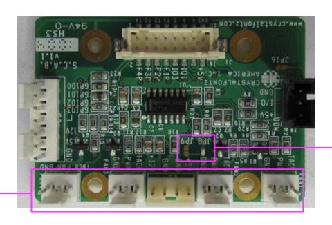
High current / Fan headers rotated 90° for easier connectivity
